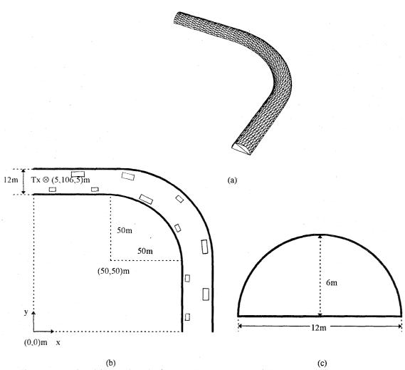
Fig. 1 A tunnel modeled by triangular facets. (a)Tunnel structure (b) Top view of the tunnel with vehicles (c) Cross section of the tunnel
