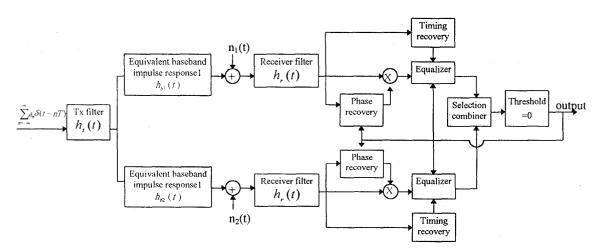
Fig. 2 Block diagram of equivalent baseband communication system with dual space antenna diversity.
